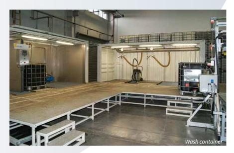
The technical container consists solely of a technical room. An entire (tank) cleaning system is built in and tested at Gröninger before being shipped, thus reducing to a minimum assembling time and costs at the client's site. The container provides a shielded, secure environment.
